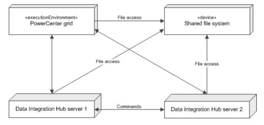
This cluster consists of two Data Integration Hub server instances, a PowerCenter environment, and a shared file system. The Data Integration Hub server instances also include the optional Managed File Transfer component. The communication lines between the Data Integration Hub servers and the PowerCenter grid represent the RMI and Web Service message flows.
