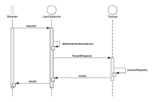
In this diagram, the browser sends the request to the load balancer. The load balancer determines which Tomcat instance will handle the request and forwards the request to the Tomcat instance. The Tomcat
