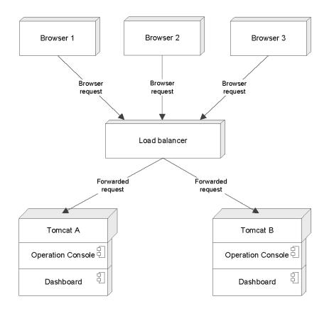
This cluster consists of three browser clients, one load balancer, and two Tomcat instances that run the Operation Console and the Dashboard. The communication lines between the components represent actions that users perform in the Operation Console that the load balancer distributes between the Tomcat instances. Synchronize the clocks of all machines in the cluster to within 30 seconds of each other to ensure proper handling of browser requests.
