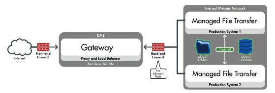
As a load balancer, Managed File Transfer Gateway spreads connections evenly across the clustered systems. This load balancing algorithm is called "round-robin", which is a common load balancing standard.
