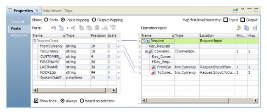
After you create input ports, map the input ports from the **Ports** area to the nodes in the **Operation Input** area. When you map an input port to a node in the operation input, the location of the port appears in the **Location** column in the **Operation Input** area.
