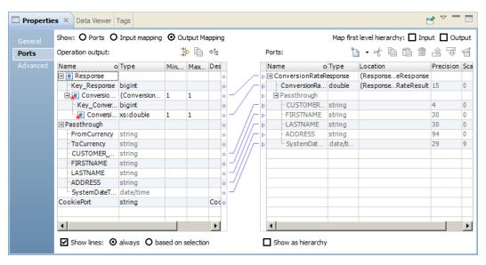
After you create output ports, map the nodes from the **Operation Output** area to the ports in the **Ports** area. When you map a node from the operation output to an output port, the location of the node appears in the **Location** column in the **Ports** area.
