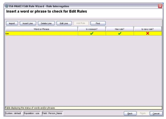
The action of committing rules via the Edit RuleWizard results in the generation of a **Local Population** ruleset. This is an ASCII text file with an extension of .ylp. Like .ysp files, .ylp files are accessible only via the Callable Routine, or one of the SSA-NAME3 GUI Clients.
