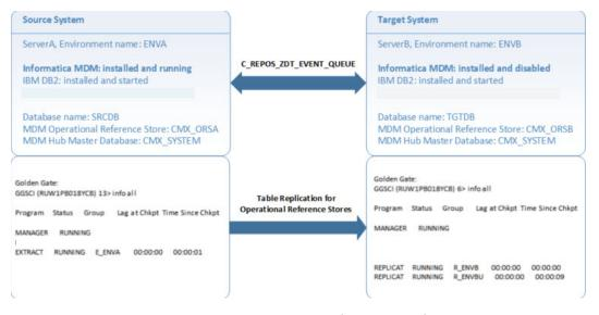
Oracle GoldenGate replicates the tables in Operational Reference Store, from the source system to the target system.
