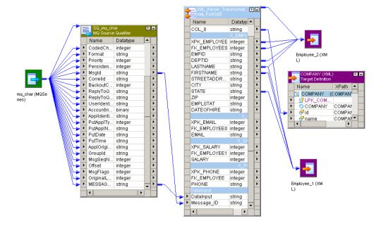
This example shows the Message\_ID port in the MQ Source Qualifier linked to the Message\_ID pass-through port in the XML Parser transformation. The XML Parser transformation passes the data through the reference output port COL0 and to the ID port in the target table.
