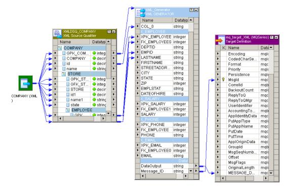
This example shows the ID data in the Source Qualifier linked to the COL0 reference input port in the XML Generator transformation. The XML Generator transformation passes the data through the Message\_ID pass-through port to the Msgld port in the target.
