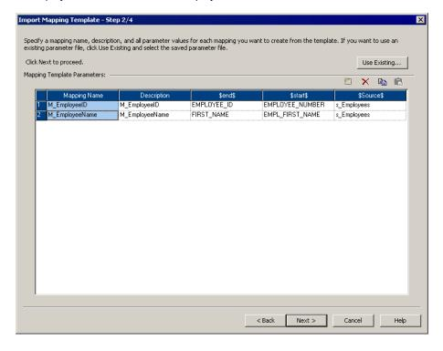
These settings create two mappings that use the same source table, but extract different data and load the data to different ports of the same target table.
