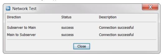
The **Network Test** dialog box shows the connectivity status for each combination of Server Manager instances. Statuses are: success and failed.
