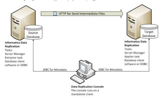
In this topology, you run the Extractor and a Server Manager instance on the source and run the Applier and a Server Manager instance on the target. The Data Replication Console optionally runs on a standalone machine.
