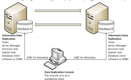
You must install Informatica Data Replication on both systems. Run an Extractor task, Applier task, and Server Manager instance on each system. You can run the Data Replication Console on a standalone system.
