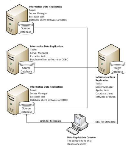
Alternatively, you can run the Extractor and Server Manager on a separate machine that can access the source database logs. Also, you can run the Applier and Server Manager on any machine that can access the target database by means of the target database connectivity client or ODBC driver. For example, run the Applier on one of the source systems. In this case, you would not install Data Replication on the target system.
