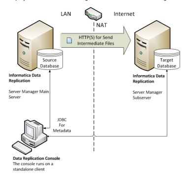
When the Server Manager Main server sends data to the Server Manager subserver on the remote system, NAT converts the IP address that is used in the LAN to a public IP address.
