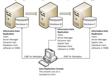
In this deployment topology, you must run a Server Manager instance on each system. Run an Extractor task on each system from which you capture database changes and replicate changes forward (Database A and Database B). Run an Applier task on each system to which you apply changes (Database B and Database C). You can run the Data Replication Console on a standalone system.
