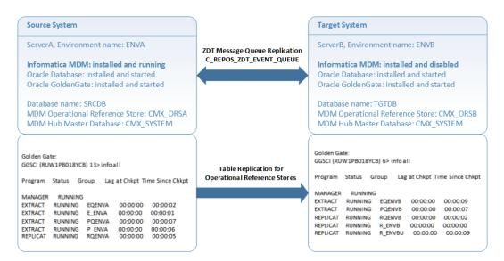
The installed versions of Multidomain MDM and the database software must be the same on the source system and the target system. The name of the MDM Hub Master Database can be different. The Operational Reference Store schema or user name can be different, but the structure of the schemas must be identical.
