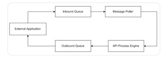
An external application sends a message containing a service invocation request to the siperian.sif.jms.queue inbound queue. The application server polls the queue for messages. The MDB of the Hub Server forwards the service request to the MDM Hub for processing. The MDM Hub processes the request and posts a response to the specified JMS outbound message queue. The external application retrieves the message from the specified message queue and processes it.
