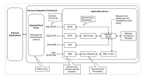
When you cannot or do not want to use the SiperianClient Java classes, you can use other access protocols to directly interact with SIF. This guide does not include information about how to directly use EJB or JMS protocols. You can use these protocols through SiperianClient if you perform any of the following tasks:
