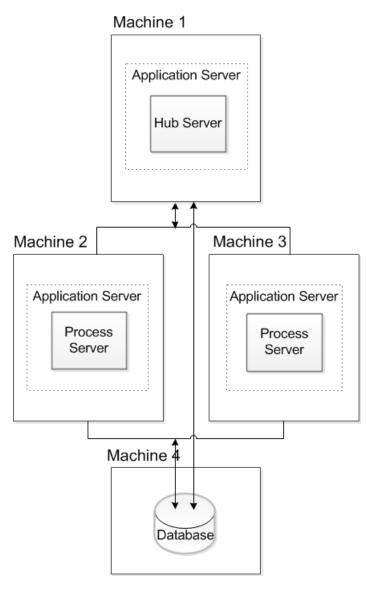
If you need high availability, you can configure additional Hub Server instances and configure external load balancers between the Hub Server instances.
