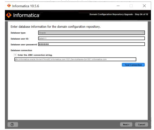
If you are upgrading a gateway node, the upgrade wizard displays the database and user account information for the domain configuration repository to be upgraded.
