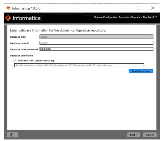
If you are upgrading a worker node, the upgrade wizard does not display the domain configuration repository information. You cannot modify the database connection information. Skip to step 21on page 90
