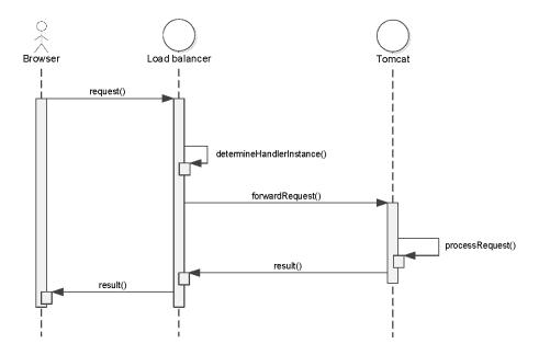
In this diagram, the browser sends the request to the load balancer. The load balancer determines which Tomcat instance will handle the request and forwards the request to the Tomcat instance. The Tomcat instance processes the request and sends the result back to the load balancer. The load balancer forwards the result back to the browser.
