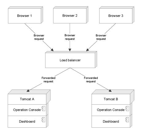
This cluster consists of three browser clients, one load balancer, and two Tomcat instances that run the Operation Console and the Dashboard. The communication lines between the components represent actions that users perform in the Operation Console that the load balancer distributes between the Tomcat
