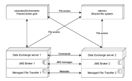
This cluster consists of two B2B Data Exchange server instances, two B2B Data Exchange JMS Broker instances, a PowerCenter environment, and a shared file system. The B2B Data Exchange server instances
