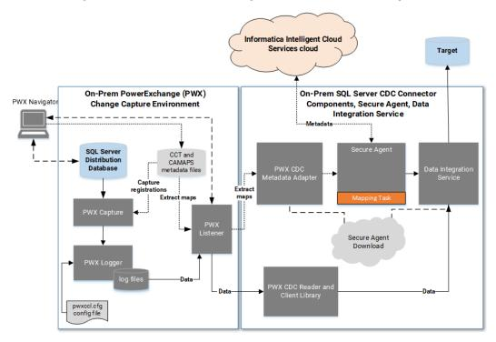
In this configuration, the PowerExchange change capture environment resides on one Windows system and the SQL Server CDC Connector environment resides on another Linux or Windows system. The PowerExchange Navigator runs on a Windows system apart from both environments. Based on this image, the following processing occurs:
