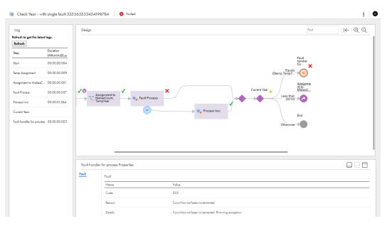
Notice that instead of the **Source** field, the **Details** field appears displaying the fault handling details that you configured for the Throw step.
