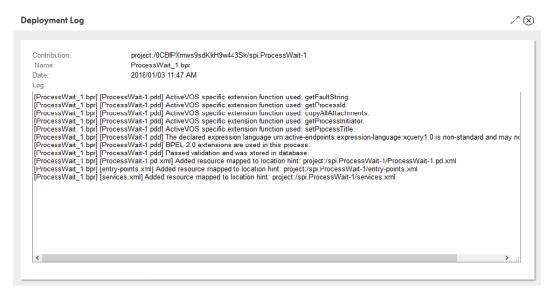
During deployment, the engine validates the deployment descriptor of the BPEL process, ensuring that the its WSDL file and other resources are available and valid for the current version of the process. If validation errors or warnings occur, make corrections and redeploy the <code>.bpr</code> file or create a new <code>.bpr</code> file for invalid processes.
