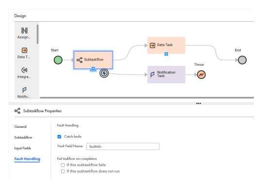
The Subtaskflow step is configured to catch faults. If a fault occurs, an email notification is sent as configured in the Notification Task step. The Throw step then stops the execution of the taskflow, returns the fault details specifying why the subtaskflow failed, and sets the taskflow status to failed. The Data Task step is not executed.
