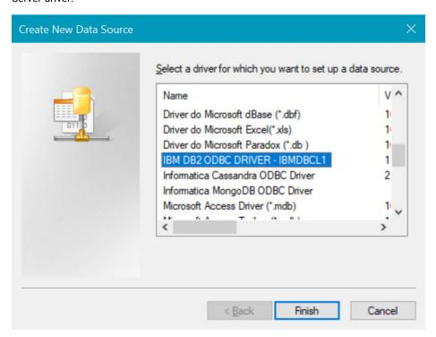
6. Select IBM DB2 ODBC driver - IBMDBCL1 to set up the data source.
