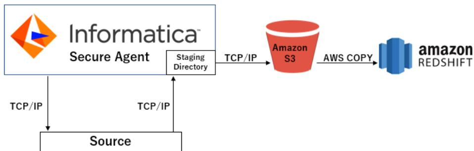
The Secure Agent reads data from a staging directory on the Secure Agent system and writes data to Amazon Simple Storage Service (Amazon S3) through a TCP/IP network. The Secure Agent then issues COPY command to write data from Amazon S3 to the Amazon Redshift target table.
