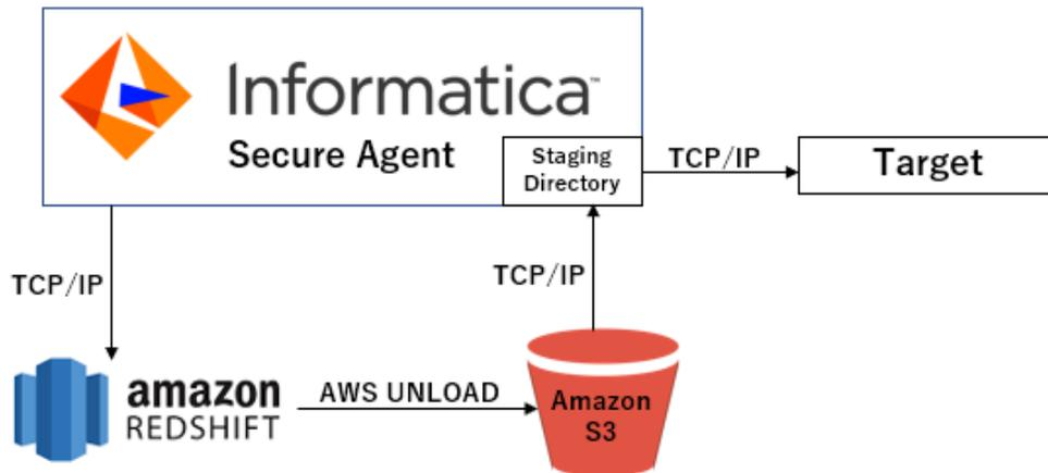
The Secure Agent connects to Amazon Redshift and issues UNLOAD command to read data from Amazon Redshift to the Amazon Simple Storage Service (Amazon S3) bucket specified in the connection properties. The Secure Agent then stores data in a staging directory on the Secure Agent system over a TCP/IP network.
