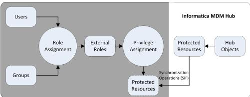
In this scenario, the MDM Hub simply exposes the protected resources using external proxies, which are synchronized with the internally protected resources using Services Integration Framework requests. All policy decisions are external to the MDM Hub.
