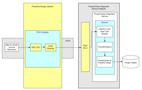
In this real-time configuration, PowerExchange CDC uses the CAPXRT access method to capture change data from DB2 for i5/OS journal receivers. The UOW Cleanser reconstructs intermingled changes read from the change stream into complete UOWs in chronological order based on end time.
