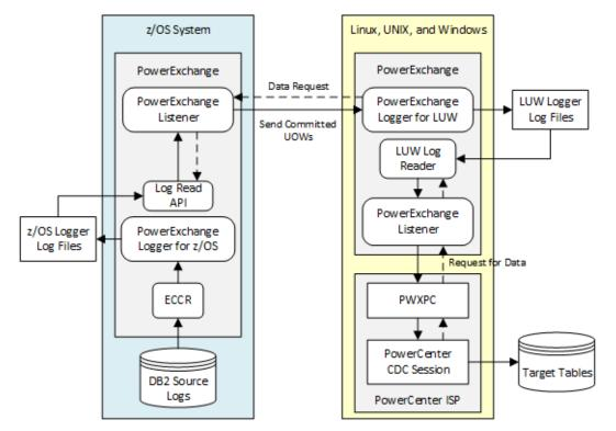
In this scenario, set the PowerExchange Logger CAPTURE\_NODE statement to point to the node name of the PowerExchange Listener on the z/OS system with the Db2 logs. Set the PowerCenter Location connection attribute to the node name of the PowerExchange Listener on the PowerCenter ISP machine where the PowerExchange Logger for Linux, UNIX, and Windows runs. Set the Map Location connection attribute to point to the node name of the PowerExchange Listener on the z/OS system.
