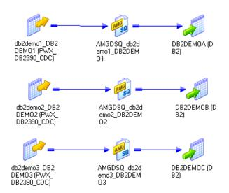
If you include this mapping in a session that uses a PWX DB2i5OS CDC application connection, PowerExchange reads the change stream and extracts changes for all three source tables in a single pass. PowerExchange extracts change data in chronological order, based on when the UOWs completed. PowerExchange passes the change data to PWXPC, and PWXPC provides the changes to the appropriate source qualifier.
