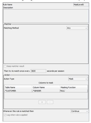
The MaskLevel0 rule uses the any rule matcher, which applies the rule to all requests that reach the MaskLevel0 rule in the rule tree. The mask rule action masks data. In the mask rule action, the NULL masking function on the GENDER column in the CUSTOMER table nullifies gender data in the result set. The continue processing action directs the request to the next rule in the rule tree.
